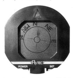
A high-precision, sensitive compass which can be used in both horizontal as well as vertical positions (push-button mode change). Any direction can be saved either before or during the flight and flown with maximum precision. The processor automatically compensates for any magnetic fields. The display is illuminated when light levels are low.
